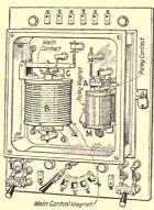
Fig. 186.-Regulator for small direct-current generators.
